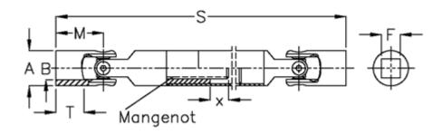
A = 25 F = 12 Longitudinal ribs = 6x11x14 M = 37 MD max N m = 20 s = 248 T = 22 x = 75
